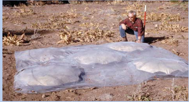
Estimates of snow water content obtained from telemetered snow sensors (snow pillows) and from manual measurement of snow courses provide the foundation for forecasting snowmelt runoff.
