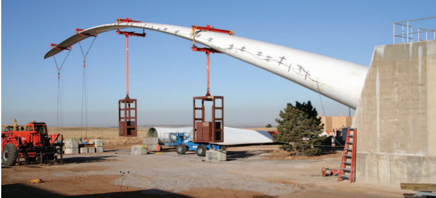
Wind Program researchers at the NWTC conduct structural tests, such as this static test on a 44-m wind turbine blade, for industry partners.
