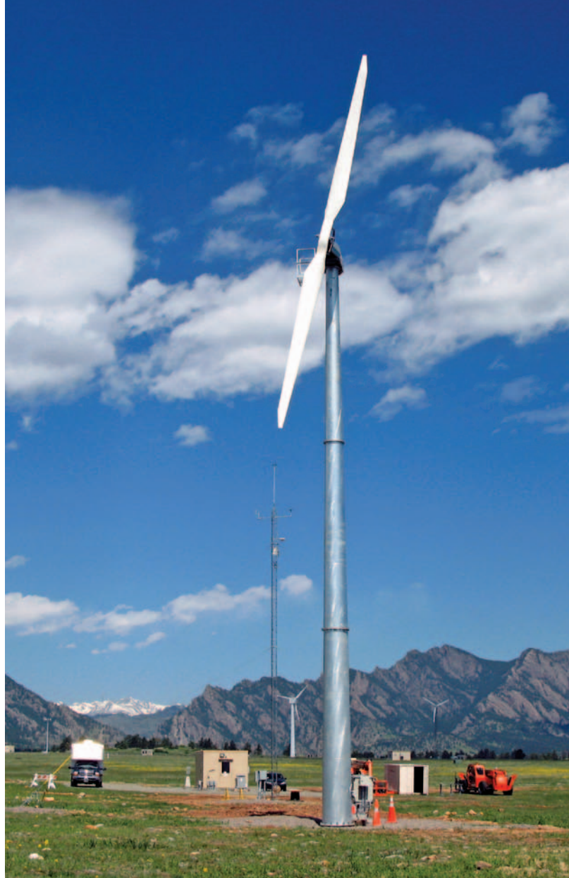
The Gaia 11-kW wind turbine is one of four wind turbines installed at the NWTC to be tested in the Small Turbine Independent Testing project.
