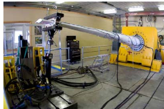
Figure 9. Fatigue testing at the A-60 Test
