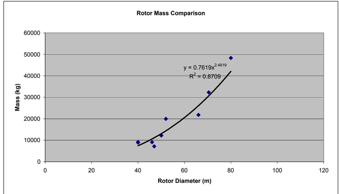
All Data for  $TSR_{Design} = 7$ ,  $C_{Max} = 8\%$  R, no parasitic weight
