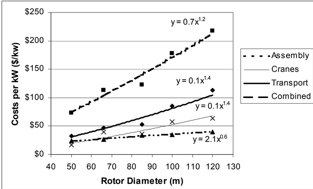
Figure 5-5. Scaling relationships by rotor diameter
