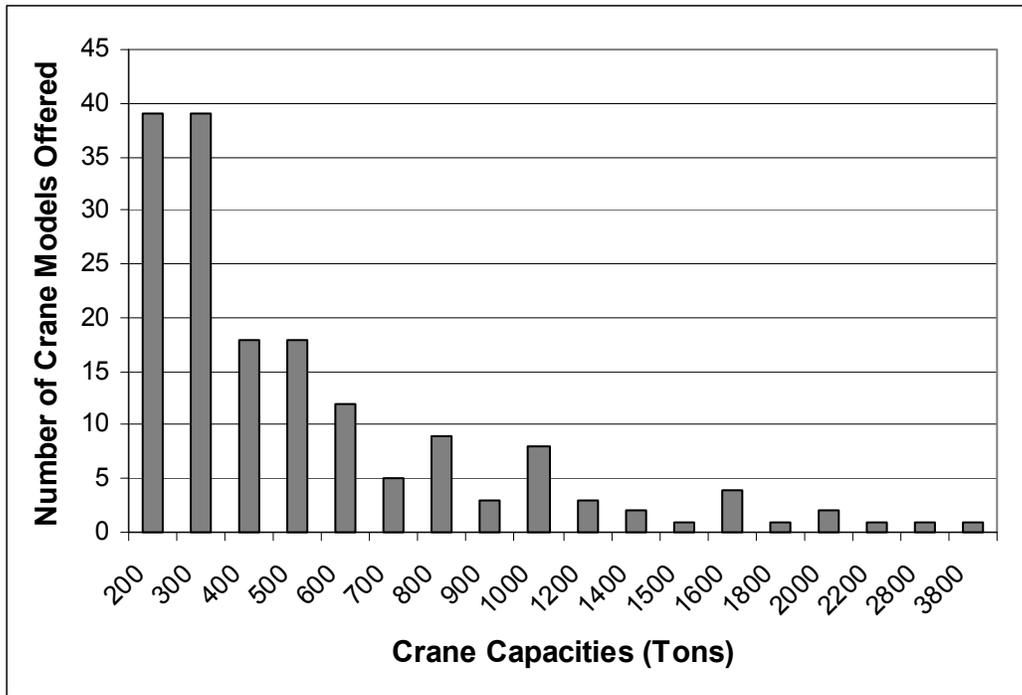
**Figure 4-12. Crane capacity trends.**
