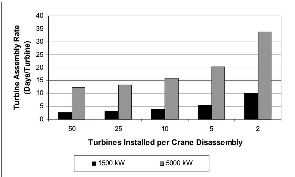
**Figure 4-16. Influence of terrain impact to turbine assembly rates**
