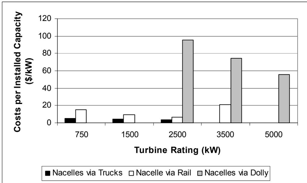
**Figure 3-6. Comparison of nacelle transport modes from Chicago, Illinois (short haul)**
