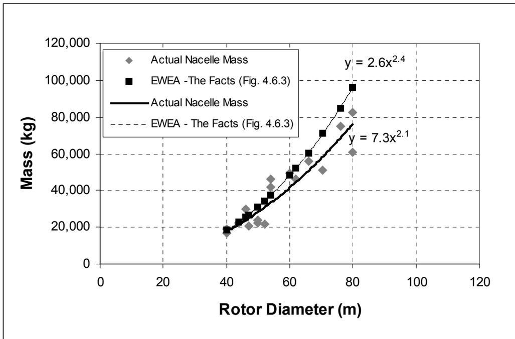
**Figure 2-2. Comparison of nacelle mass equations**
