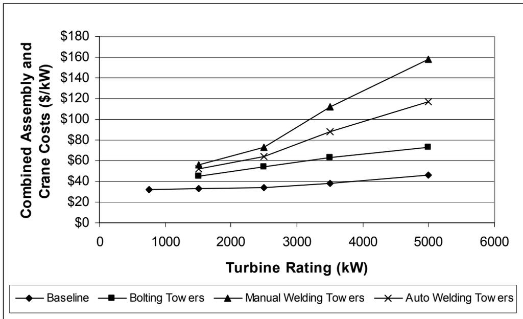
**Figure 4-14. Combined assembly and crane costs by scenario**
