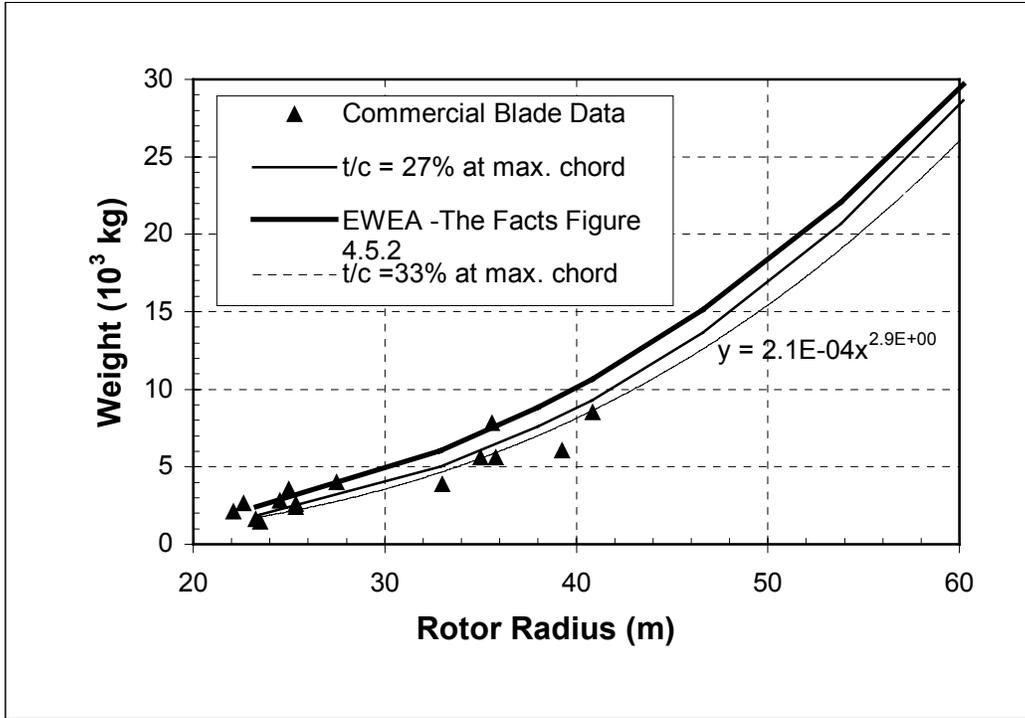
**Figure 2-1. Comparison of blade mass equations**
