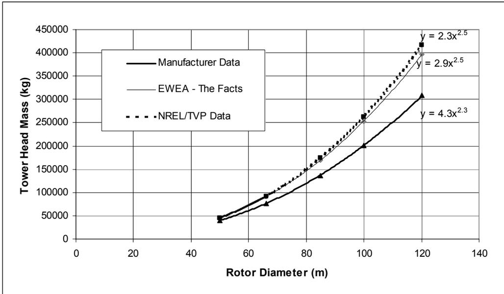
**Figure 2-3. Comparison of tower head mass equations**
