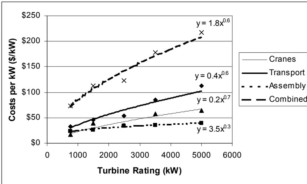
Figure 5-6. Scaling relationships by turbine rating
