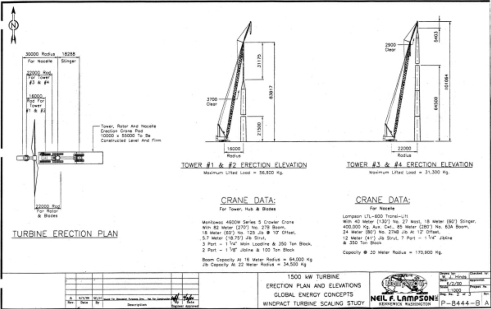
Figure 4-2.1500 kW crane
