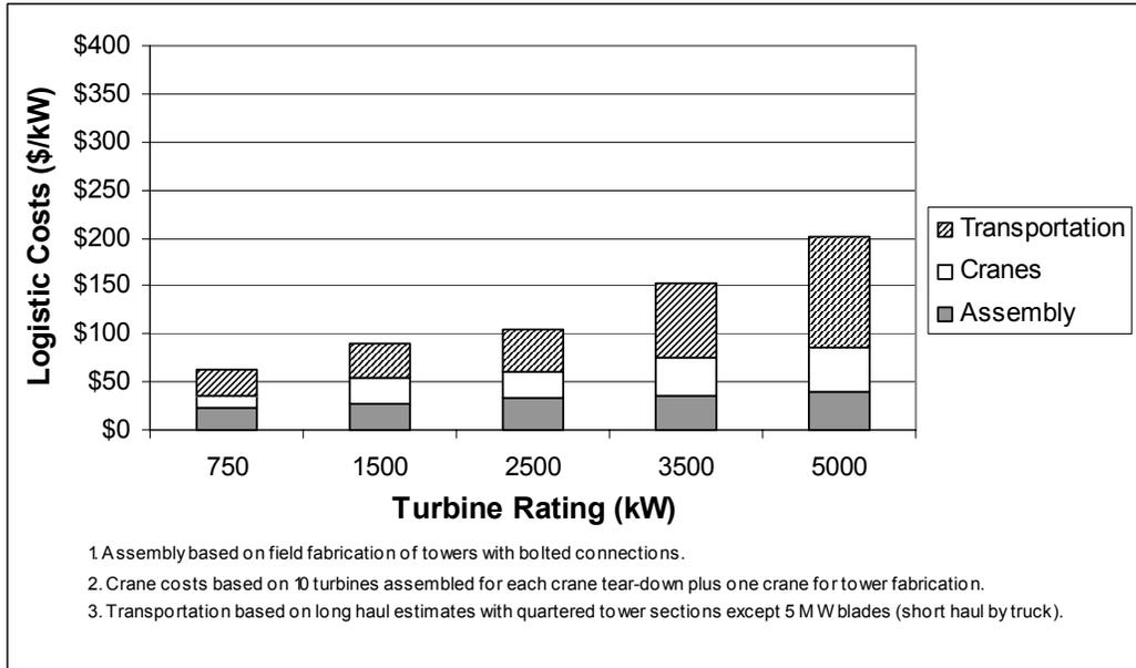
**Figure 5-4. Logistic costs for multi-megawatt turbines in South Dakota**
