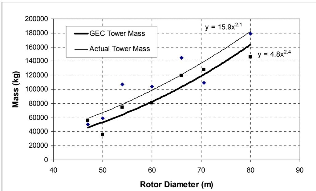
**Figure 2-4. Comparison of tower masses**
