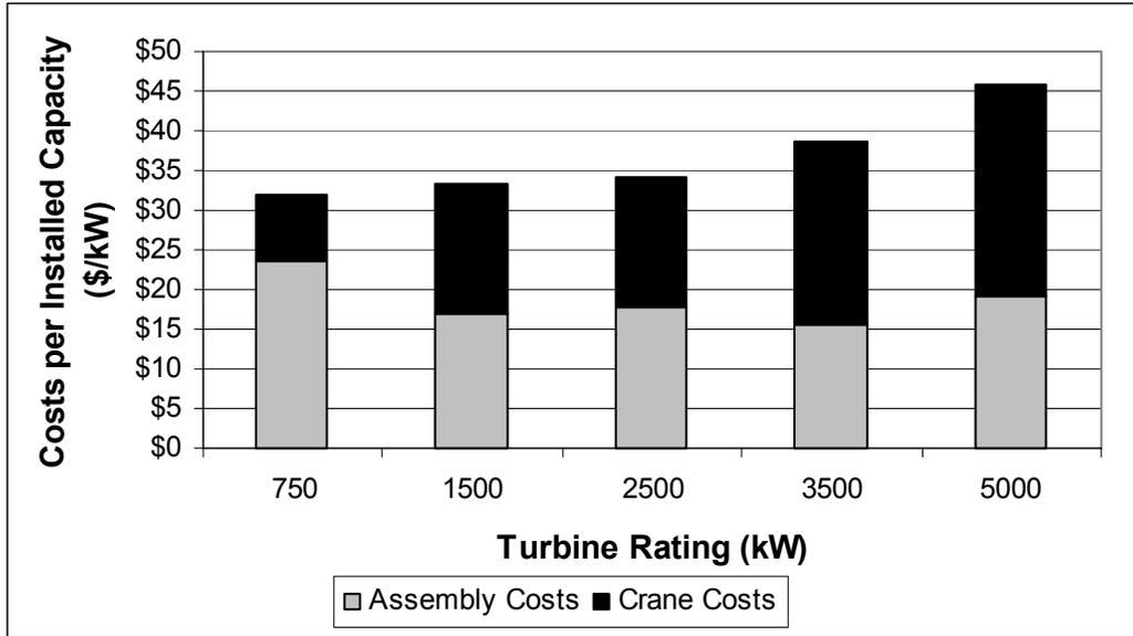
**Figure 4-6.Scenario 1 assembly and crane costs**
