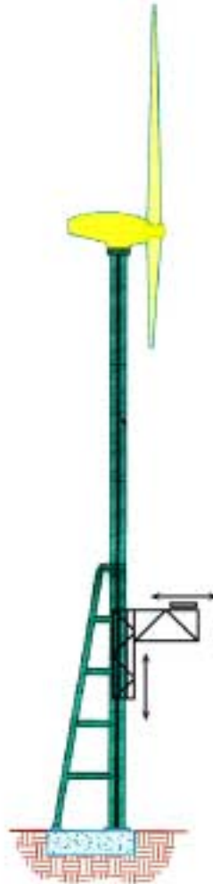
Figure 13. Valmont Tower with Self-Erection Sled
