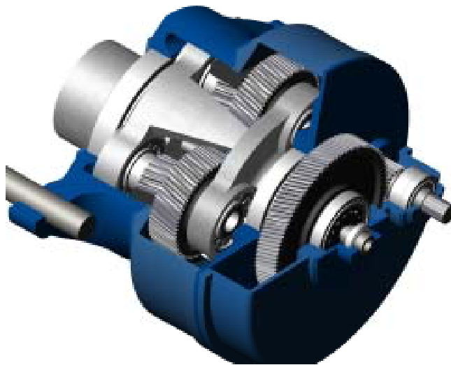
Figure 7-2. A 1.5-MW compound planetary helical gearbox.
