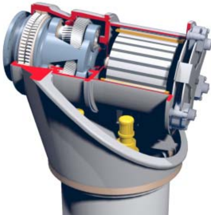
Figure 7-18. A 1.5-MW MS-1 (gearbox and housings cutaway).
