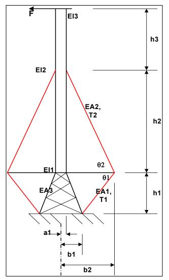
Figure 2-1. Two-dimensional layout of hybrid tower.
