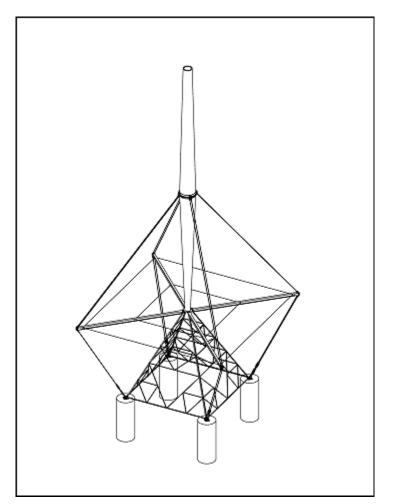
Figure 1-1. Representative stayed tower configuration.
