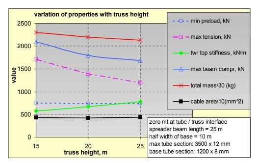
Figure 3-6. Variation of key properties with truss height.
