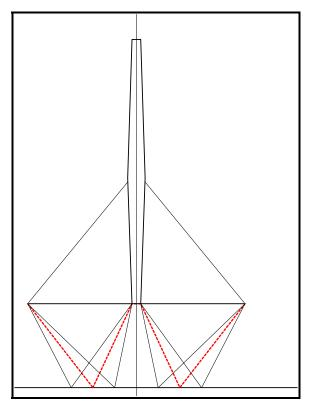
Figure 3-2. Outlines of Group #2: variation of truss base width.
