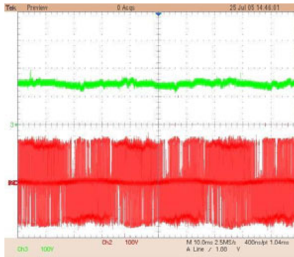
Figure 4.12: Waveforms of a capacitor voltage and an output PWM line-line voltage with capacitor voltage regulation
