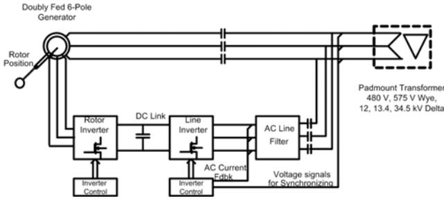
Fig. 3. Conceptual block diagram of WECC Type 3 WTG
