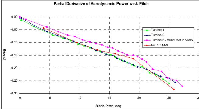
Fig. 6.  $dP_{\text{mech}}/d\theta_{\text{pitch}}$  as a function of  $\theta_{\text{pitch}}$  for example Type 3 and 4 WTGs
