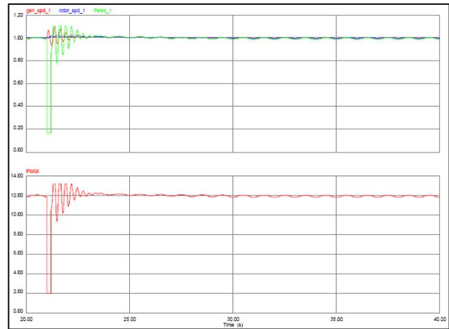
Fig. 12. Single and multiple WTG power output, same mainshaft wind-up
