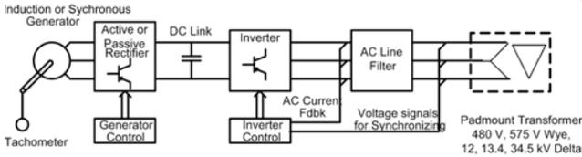
Fig. 4. Conceptual block diagram of WECC Type 4 WTG
