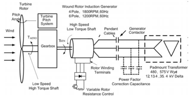
Fig. 2. Conceptual block diagram of WECC Type 2 WTG
