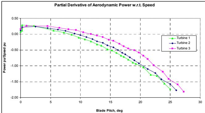
Fig. 7.  $dP_{\text{mech}}/d\omega_{\text{rotor}}$  as a function of  $\theta_{\text{pitch}}$  for example Type 3 and 4 WTGs
