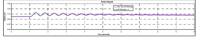
Fig. 9. Time response of  $\omega_{\text{rotor}}$  with and without  $dP_{\text{mech}}/d\omega_{\text{rotor}}$  term
