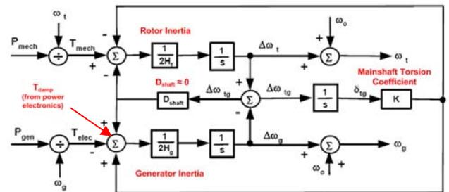
Fig. 10. Two-mass, compliant-shaft drivetrain representation
