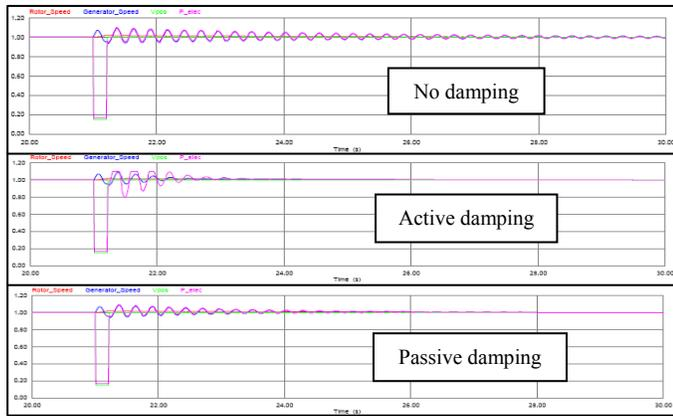
Fig. 11. Time domain response of two-mass, compliant-shaft drivetrain with three different mainshaft mode damping models
