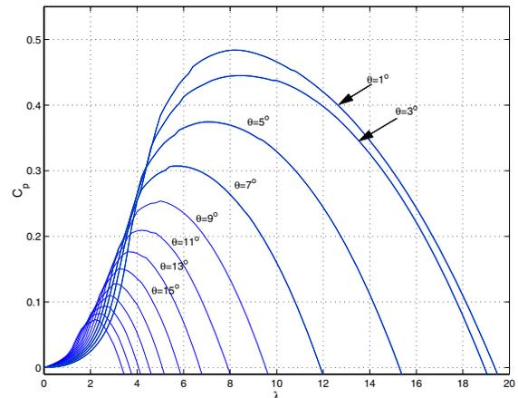
Fig. 5. Typical  $C_p$  curves for variable-speed, variable-pitch WTG
