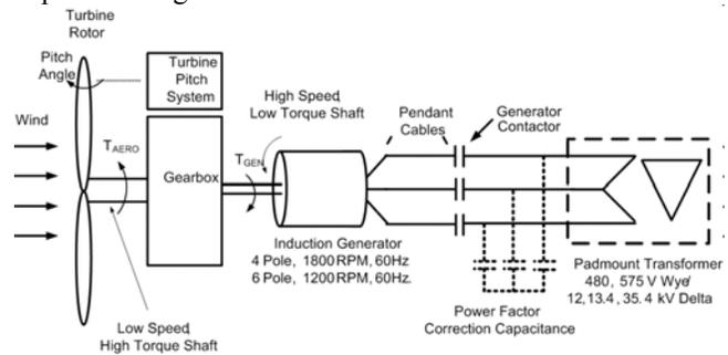
Fig. 1. Conceptual block diagram of WECC Type 1 WTG
