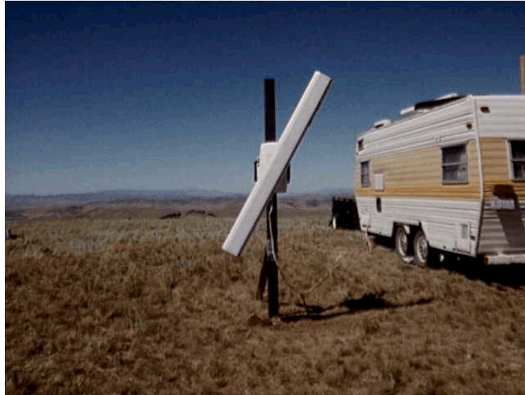
Figure 3. Positioning of radar antenna for detection of flight altitude of birds, Norris Hill Wind Resource Area, Madison County, Montana. View is to north.
