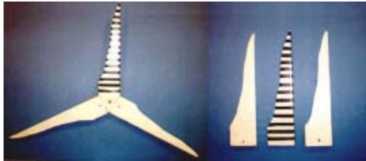
Figure 11. Blade pattern 3. One blade, all thin stripes; two blank blades.
