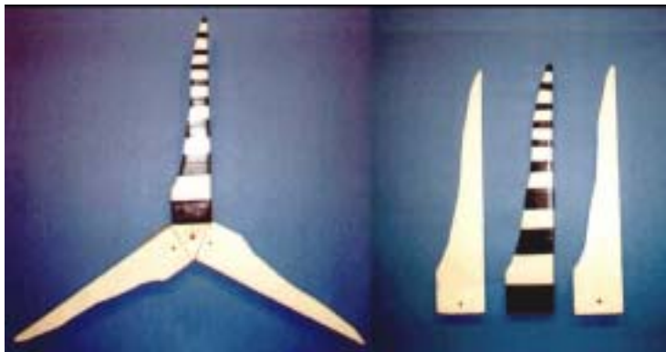
Figure 14. Blade pattern 6. One blade; thick stripes at the inner half of the blade and thin stripes at the outer half; two blades blank.
