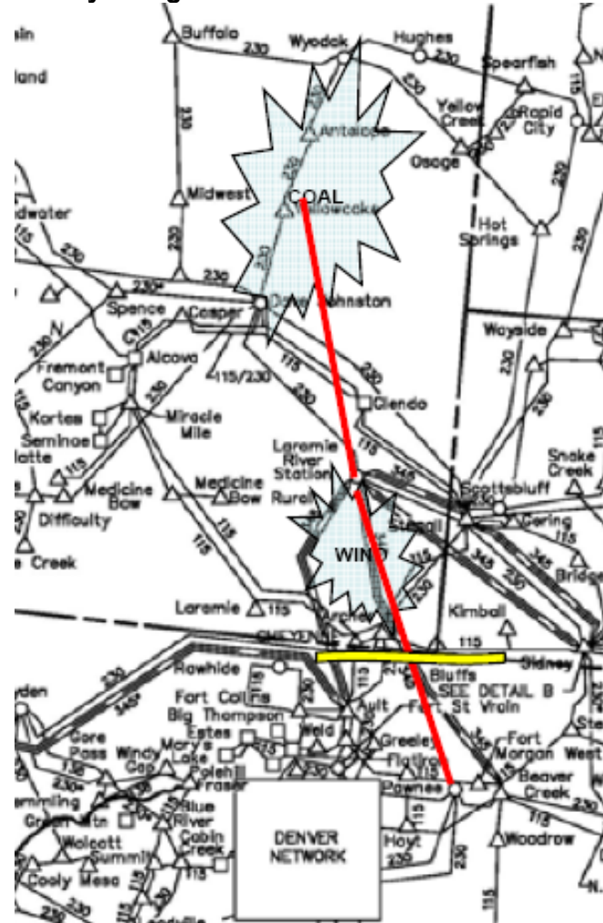
Figure 3. Wyoming-Colorado Intertie Transmission Project
